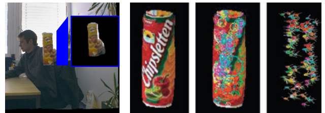
Fig. 6. Spatial segmentation for object learning (left), side view of an object, detected feature points and corresponding feature point cloud (right three images)
